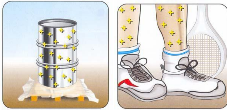
Fig. 1 Examples of electrostatic charges [1] left: metal drum on insulated base / right: person with insulated footwear
